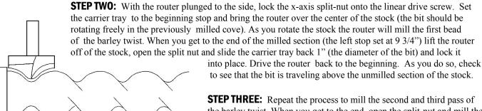
**STEP THREE:** Repeat the process to mill the second and third pass of the barley twist. When you get to the end, open the split-nut and mill the second cove (Fig B). Release the tailstock, remove the workpiece and insert the second leg into the mill. Repeat steps 1-3 for all 4 legs.
